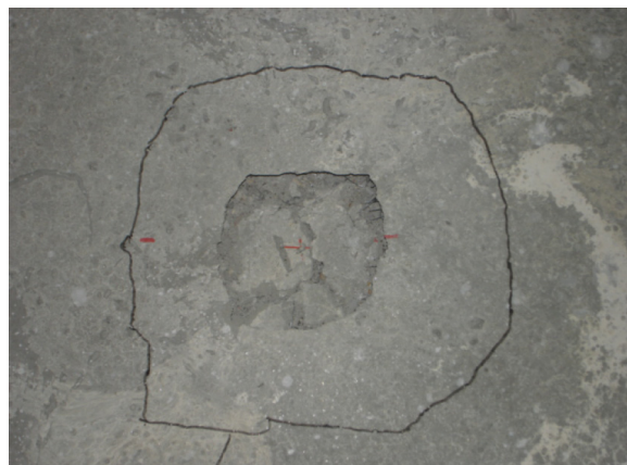
Figure 10. Punching critical contour.
