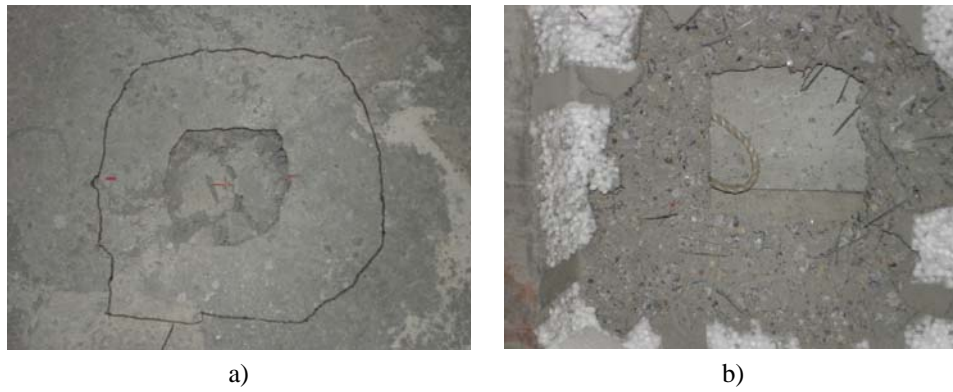
Fig. 13 -- Punching critical contour: a) top, b) and bottom faces.
