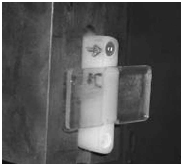
Figure 6. PET overmoulded onto a SL Huntsman 5260 block.
