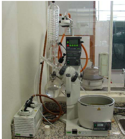
Figure 4. Rotary Evaporator (University of Minho) used to recover the bitumen
