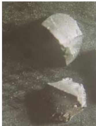
Figure 3. Crumb rubber obtained from cryogenic process
