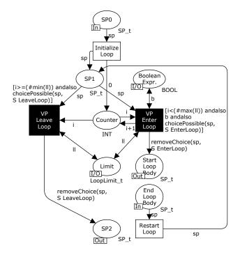
Figure 7. The CPN module for modelling loops.
