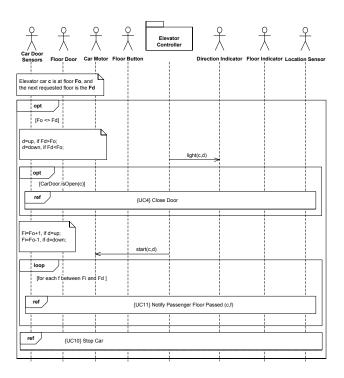
Figure 2. SD for main scenario of UC2 Service Floor.
