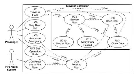
Figure 1. The UC diagram for the Elevator Controller.
