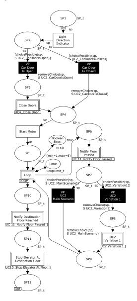
Figure 5. CPN module for UC2's main scenario.
