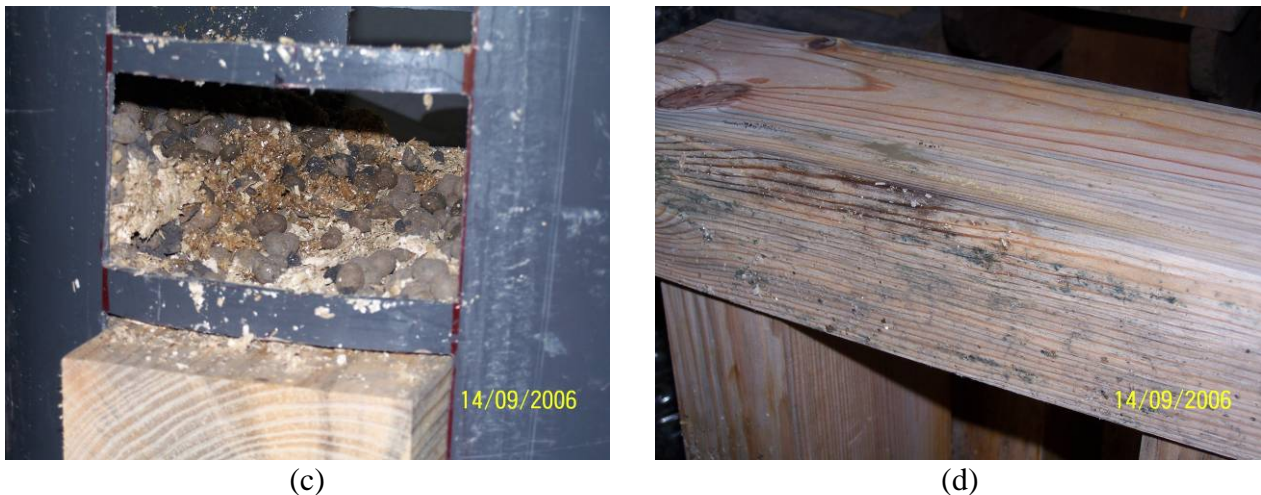
Fig. 16: Decay tests currently running on LNEC: (a, b) mounting of a decay column; (c) Detail of the mixture used to fill the tube; (d) incipient decay detected in some test specimens
