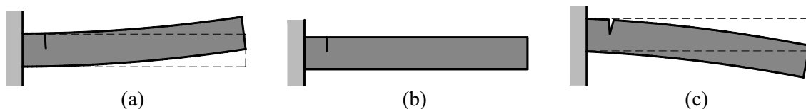
Figure 1: Crack breathing of a cantilever beam: (a) crack closed with restoration of the initial stiffness; (b) transitory stage; and (c) crack open with minimum stiffness
