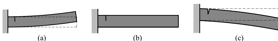
Figure 1 : Crack breathing of a cantilever beam: (a) crack closed with initial stiffness; (b) transitory stage; and (c) crack open with minimum stiffness.
