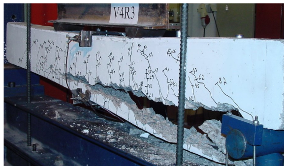
Figure 10. Typical failure mode of a strengthened beam after its failure (beam V4R3)
