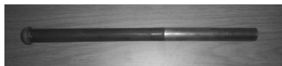
Figure 3. Two-piece rod made of iron and nylon
