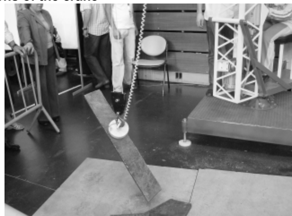
Figure 6. Electromagnet elevating an iron piece
