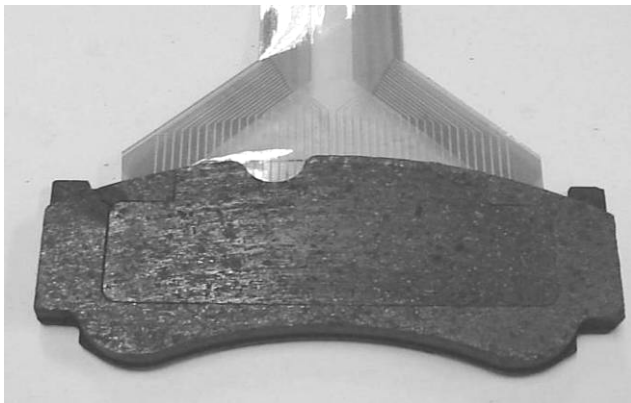
Figure 8 – View of pad with embedded pressure film.
