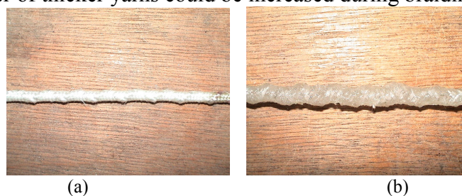
(a) braided fabric (b) braided reinforced composite rod
