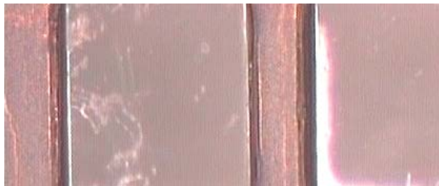
Fig 6: Metal pads before removal of SU-8 sacrificial layer.
