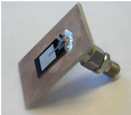
Fig. 3. A photo of the patch antenna fabricated on a HRS wafer, already mounted for measurements.
