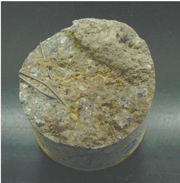
Fig. 5. Detail of the failure mode verified in one test of the model B1C1 with bond coat P2.
