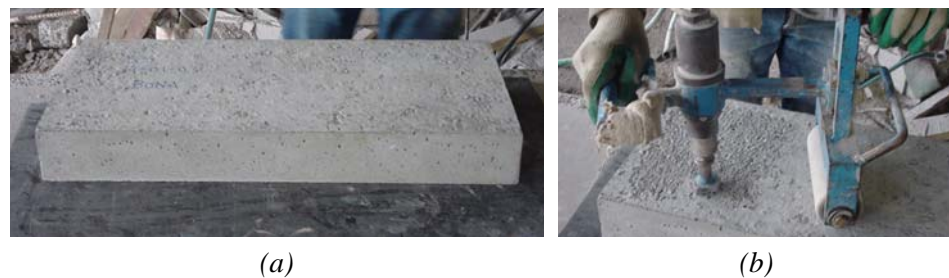
Figure 2: The specimen surface before roughening (a) and the roughening machine (b).
