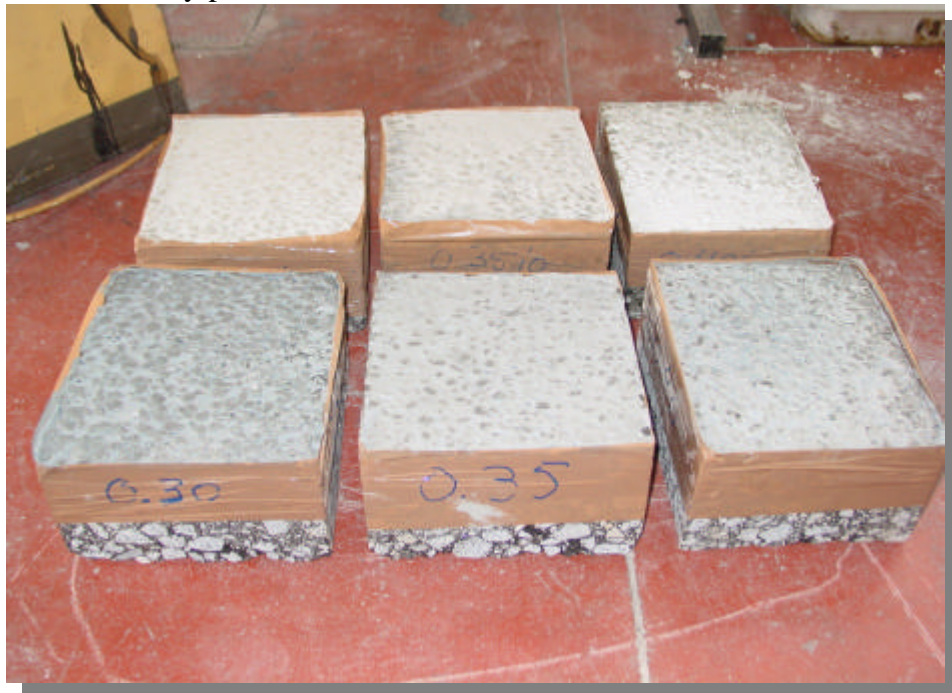
Figure 3 – Slabs filled with cement grout
