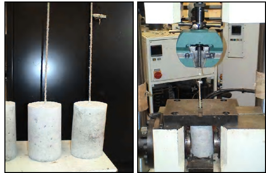
Fig. 4. Samples for adherence test
