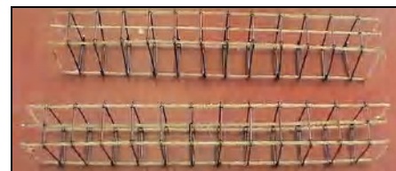
Fig. 6. Composite rods reinforcements used
