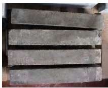
Fig. 8. Concrete beams reinforced by composite rods
