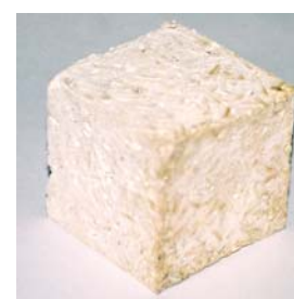
Fig. 1 - Concrete with Cellulose of Industrial Hemp (hemp hurds) – University of Minho
