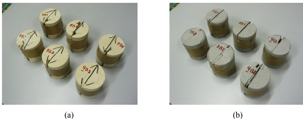
Figure 5.9 – Failure patterns for the tension tests: (a) Noto specimens and (b) Serena specimens.
