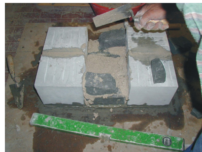
Figure 5.1 – Wallets dimensions in mm: (a) straight collar joints and (b) keyed collar joints.
