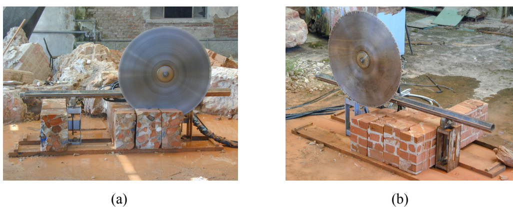
Figure 4.4 – Preparation of the specimens recovered from the ruins of the Pavia Civic Tower: (a) PRu and (b) PRe .
