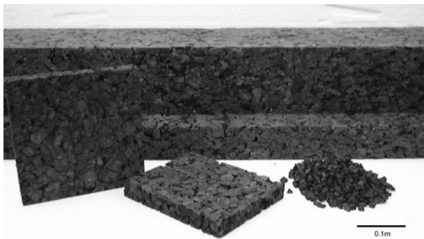
17 Some of different shapes of insulation corkboard and regranulated ICB
