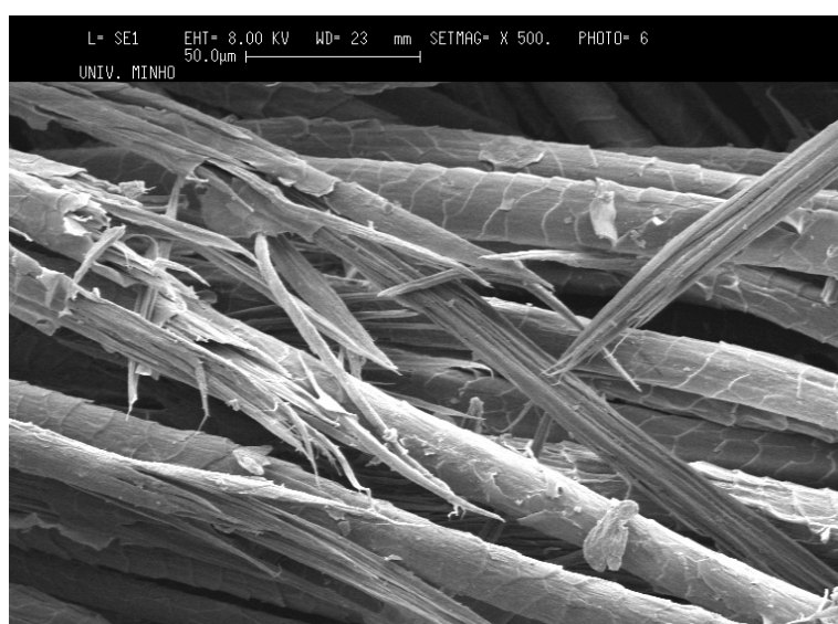
Figure 2.1 – SEM microphotography showing damaged and undamaged wool fibres after treatment with Subtilisin, in pH 7.6 buffer, at 37°C, for 3 days.
