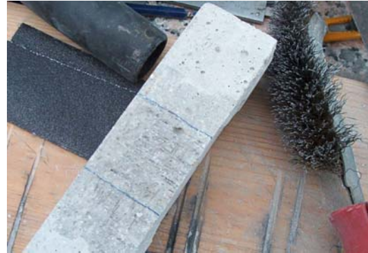
Fig. 2 – Specimen after surface preparation.
