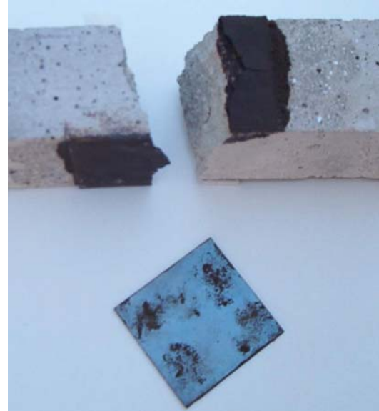
Fig. 10 – Adhesive failure of a specimen.
