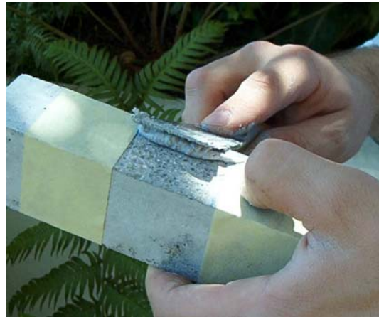
Fig. 3 – Application of epoxy on a specimen.
