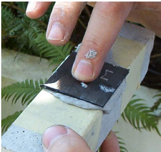
Fig. 5 – Bonding a CFRP plate to a mortar specimen.
