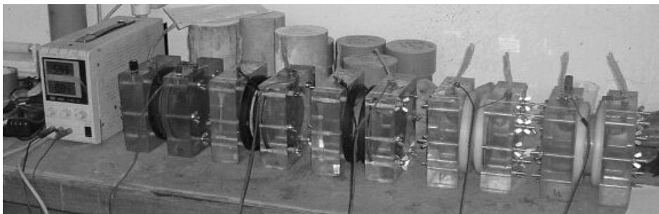
Figure 5. Tests apparatus for the evaluation of the concretes ability to resist chloride penetration (ASTM C1202).
