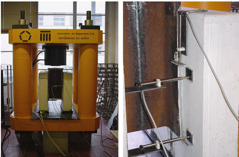
Fig. 5. Push-out test setup and measurement settings.
