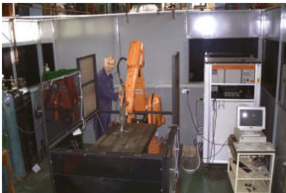
1 Setup for Rapid Prototyping using Robot Welding
