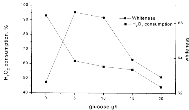
Fig. 3. Peroxide consumption (initial H 2 O 2 concentration 0.4 g/liter) and bleaching effect in the presence of glucose in the bleaching bath.
