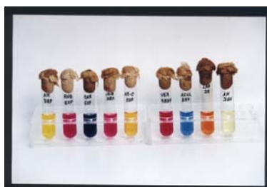
Figure 5. Decolorization tests of commercial textile dyes by UM45 in IDM. (a) Initial aspect; (b) after 18-24h incubation
