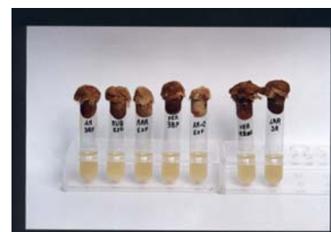
Figure 5. Decolorization tests of commercial textile dyes by UM45 in IDM. (a) Initial aspect; (b) after 18-24h incubation
