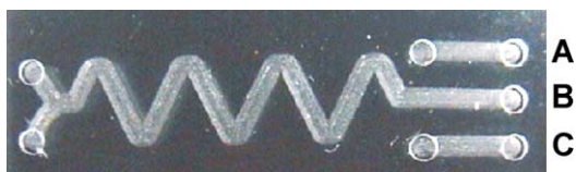
Fig. 3. The fluidic channels. It comprises three fluidic channels. Channel A is needed to obtain the baseline reference and to calibrate the light source. Channel B allows the mixed solution analysis (reagent plus sample). Channel C is needed to calibrate the biochemical substance concentration (well-known biochemical calibrator).
