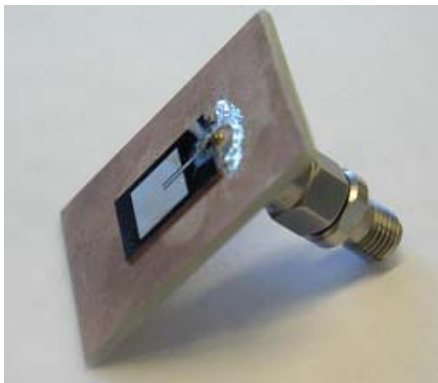
Fig. 5: Patch antenna fabricated on a high resistive silicon substrate, already mounted for measurements.
