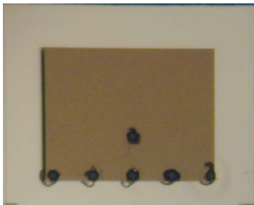
Figure 4. Photograph showing detail of the bottom glass substrate with the 200 \mu\text{m} diameter ablated vias and the patterned middle Al antenna patch.
