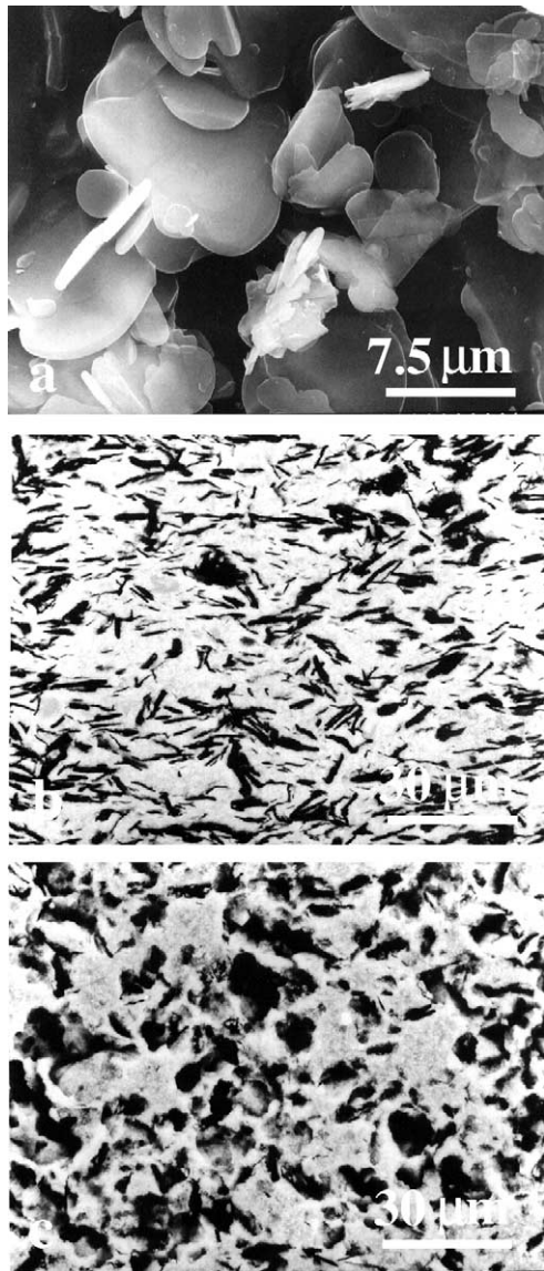
Fig. 1. SEM micrographs of (a) BN platelets; unworn surfaces of \text{Si}_3\text{N}_4 -25 vol.% BN composites in perpendicular (b) and parallel (c) planes to the sliding motion.
