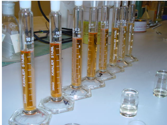
Figure 6.2 – Colour changes according to chloride concentration.
