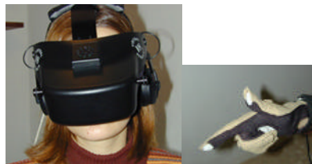
Figure 2: HMD and a paradigm for the virtual pointer (using a virtual glove)
