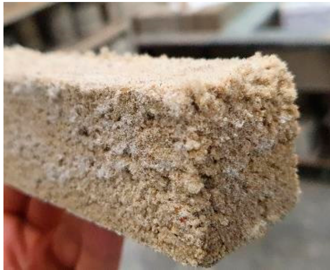
Figure 8. Efflorescence caused by sodium carbonate precipitation on the surface of N14S0 WGR specimen.
