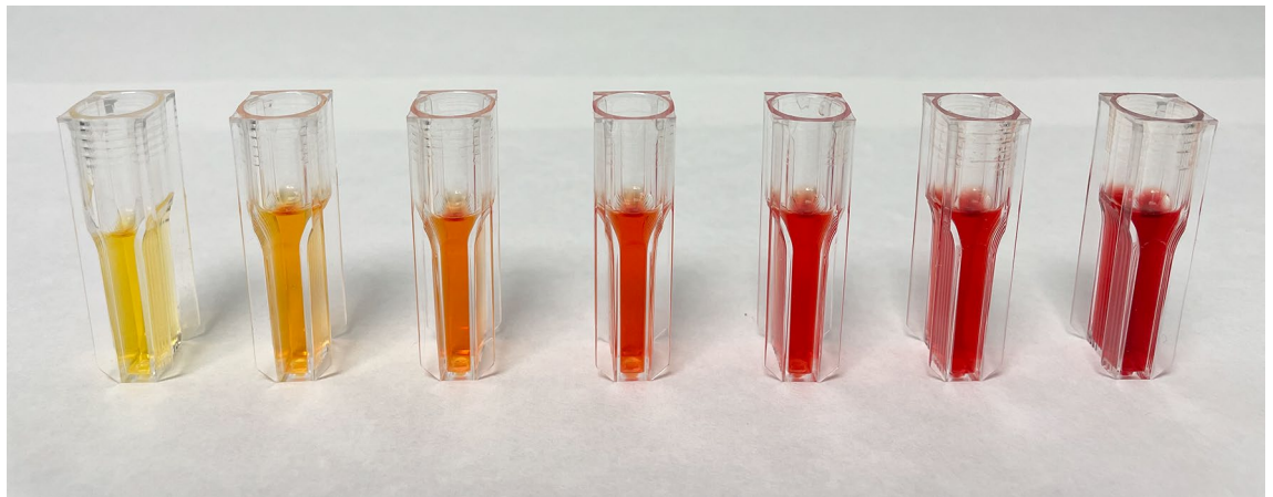
Figure 1. Color of serum samples containing different haemoglobin (Hb) concentrations (from the left to the right: 0.0, 0.2, 0.5, 1.0, 2.5, 5.0 and 10 g L -1 , respectively). (Taken in our laboratory at the Faculty of Veterinary Medicine of the University of Santiago de Compostela on May 24, 2022 by C. Herrero Latorre using an Apple Iphone 12).
