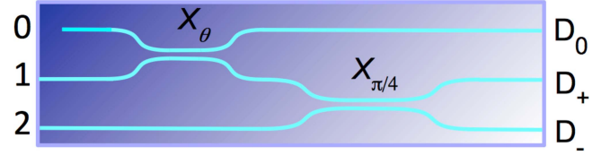
Fig. 2. Drawing of an integrated quantum optical circuit for implementing a POVM for states |L_{\pm}\rangle = \cos \alpha |1_1\rangle \pm i \sin \alpha |1_2\rangle .
