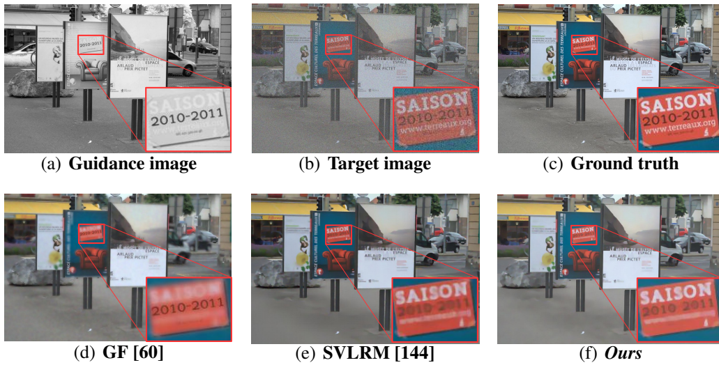
Figure 36: Joint denoising result ( \sigma = 25 ) on RGB/NIR. Our filter better preserves finer details with fewer noises.
