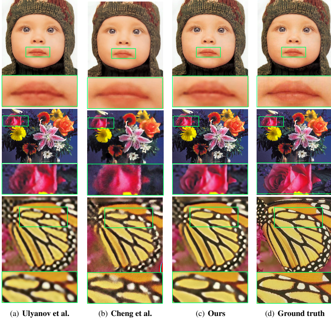
Figure 17: Super-resolution. Results on the ‘baby’ image and the ‘flowers’ image for 4 \times super-resolution, and on the ‘butterfly’ image for 8 \times super-resolution. From the regions masked by the green rectangles, we observe our method is able to better recover details with fewer artifacts (best viewed digitally).
