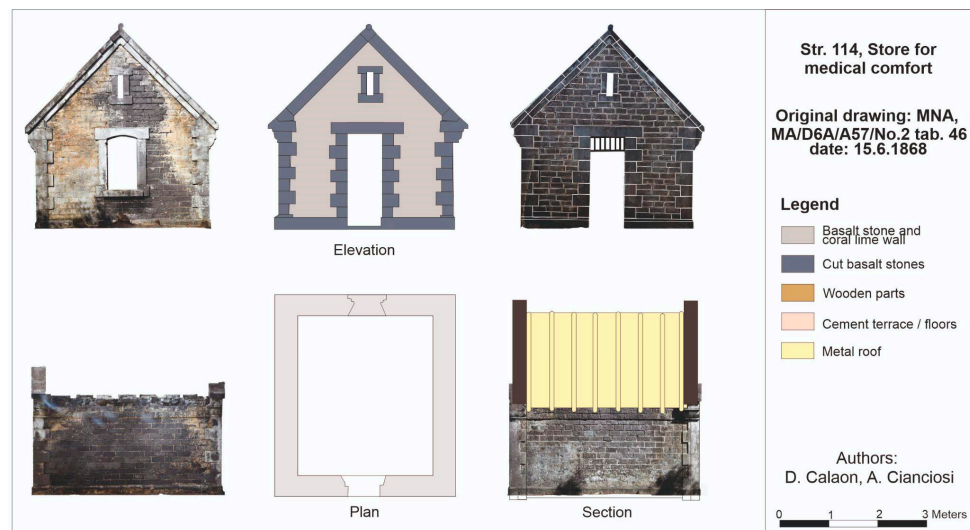
Figure 10. The store for medical comfort: photogrammetric orthomosaic image and redrawn archival architectural plan.
