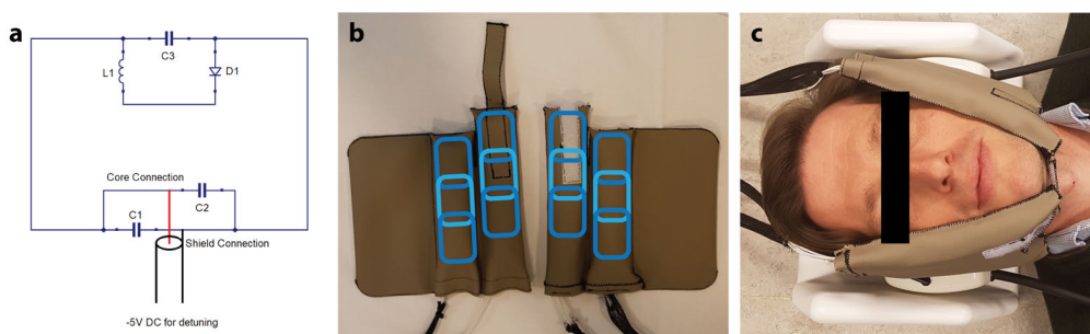
FIGURE 5.1 — Design and lay-out of the flexible coil: a: The schematic of a single coil element with three capacitors (C1-3), one inductor (L1), and one diode (D1). b: Three of these elements were assembled in a phased array indicated by the blue rounded rectangles. c: The coil was placed directly on the cheeks of a subject. The synthetic leather strap and flaps, which were placed between the headphones and the subject's head, kept the coil in position. The white 3D-printed headrest minimised head rotation during scanning.
