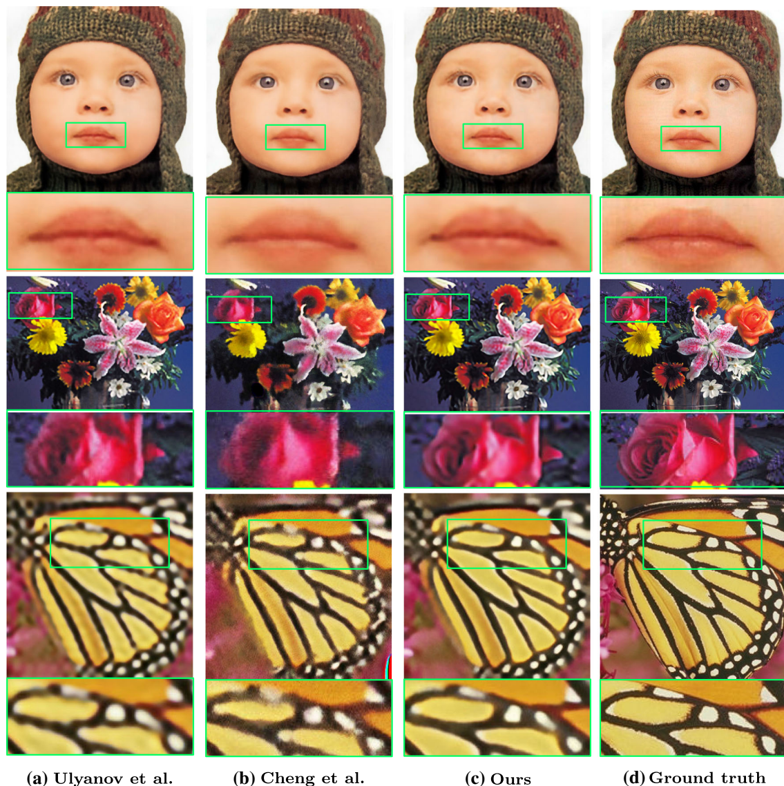
Fig. 15 Super-resolution. Results on the ‘baby’ image and the ‘flowers’ image for 4\times super-resolution, and on the ‘butterfly’ image for 8\times super-resolution. From the regions masked by the green rectangles, we observe our method is able to better recover details with fewer artifacts (best viewed digitally)
