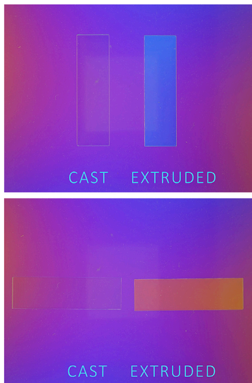
Figure 5. Cast and extruded PMMA viewed through the Strain Viewer
