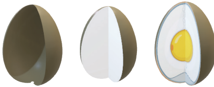
Figure 1. The difference between a surface model, solid model, and volumetric model of an egg.
