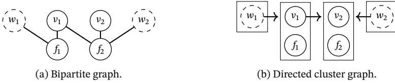
Figure 4.3: The bipartite graph in Figure (a) is associated with the constraints in Example 4.4. Exogenous variables are indicated by dashed circles. The directed cluster graph that is obtained by applying Algorithm 1 is shown in Figure (b).
