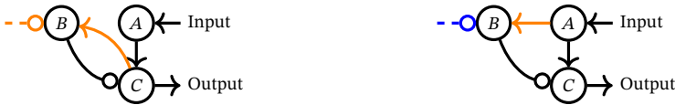
(a) Negative feedback with a buffer node. (b) Incoherent feedforward loop with proportioner node.
