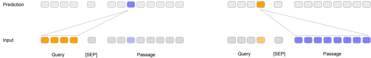
Figure 1: RelEmb pre-training task. Predicting randomly tokens in the passage from the query (left) or tokens in query from the passage (right).
