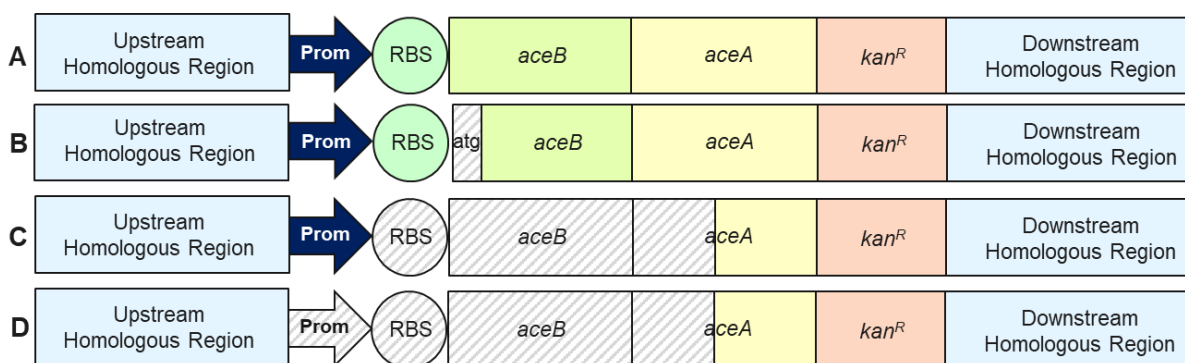
Figure 3.6 Schematic representation of the deletions (grey area) found in LIB- \Delta fumC \Delta zwf (A, B, C, D) and LIB- \Delta fumC (A, B, D). (A) Intact cassette. (B) Deletion of the start codon (atg) of the MS gene ( aceB ). (C) Deletion of the RBS, the MS gene ( aceB ) and part of the ICL gene ( aceA ). (D) Deletion of the promoter, the RBS, the MS gene ( aceB ) and part of the ICL gene ( aceA ).
