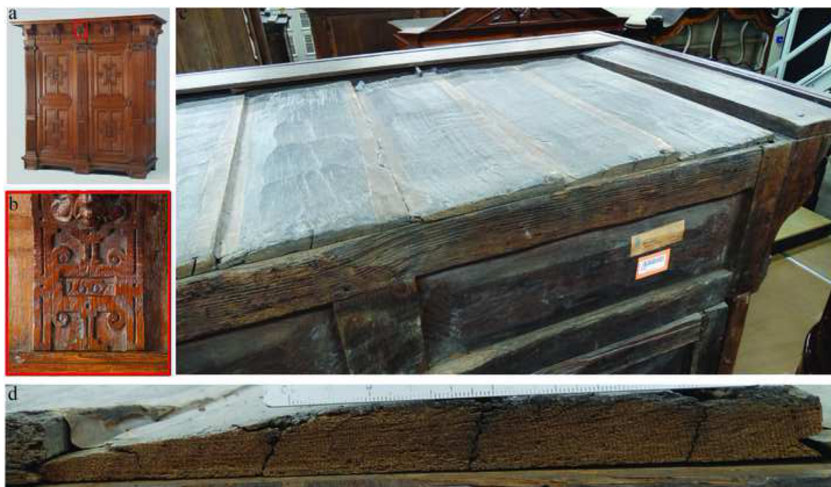
Fig. 1. Cabinet from the Rijksmuseum (Amsterdam) collection ( http://hdl.handle.net/10934/RM0001.collect.55023 ). The cabinet is made of oak and signed in 1607 (a, b). Dendrochronological research has determined that the top planks are made of Baltic oak (c). Those planks illustrate the high-quality timber products (i.e. radial planks cleft from slow grown trees) that were imported into the Netherlands in the early 17th century (d; second plank from the right on (c)). Source photos: a, b, Rijksmuseum; c, d: Marta Domínguez-Delmás.
