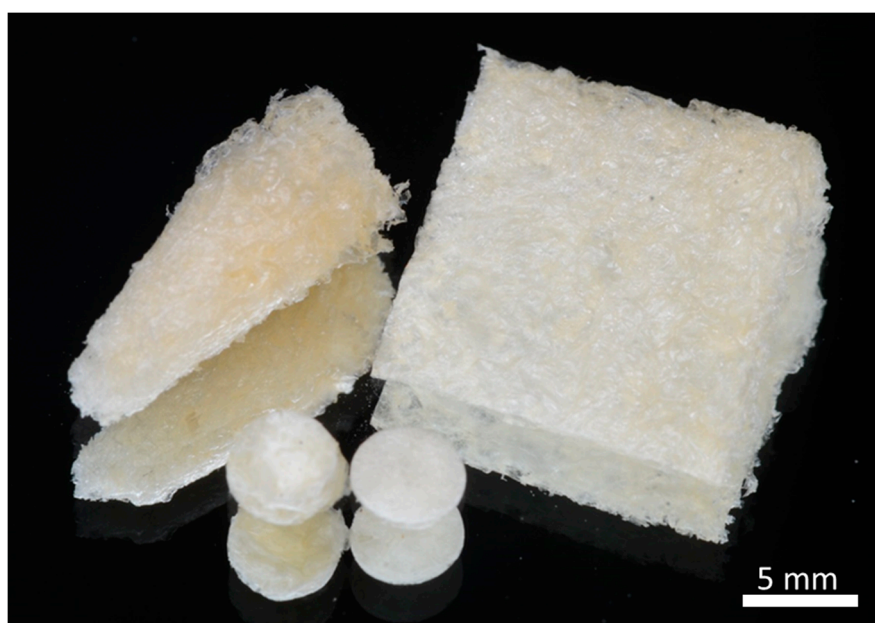
Figure 6. The fabricated CS-DA scaffold after freeze-drying.
